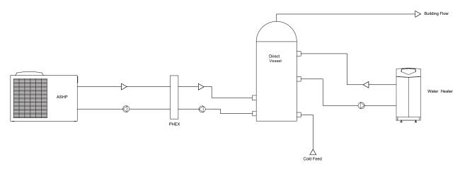
Amicus HT air source heat pump providing hybrid hot water solution, with EcoKnight gas-fired condensing water heater
