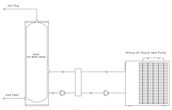
Stand-alone Amicus HT air source heat pump providing hot water only
